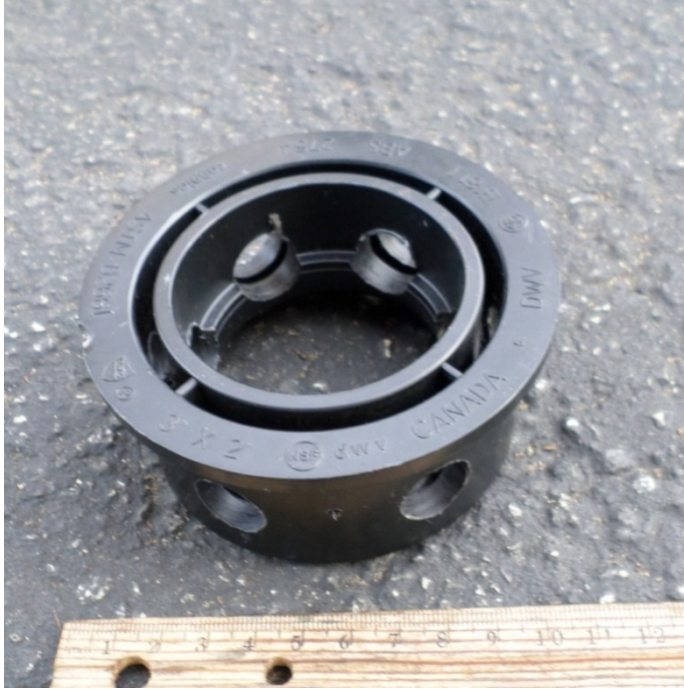
RANGER prop build photo #21: ABS flange with holes drilled through the side wall.
