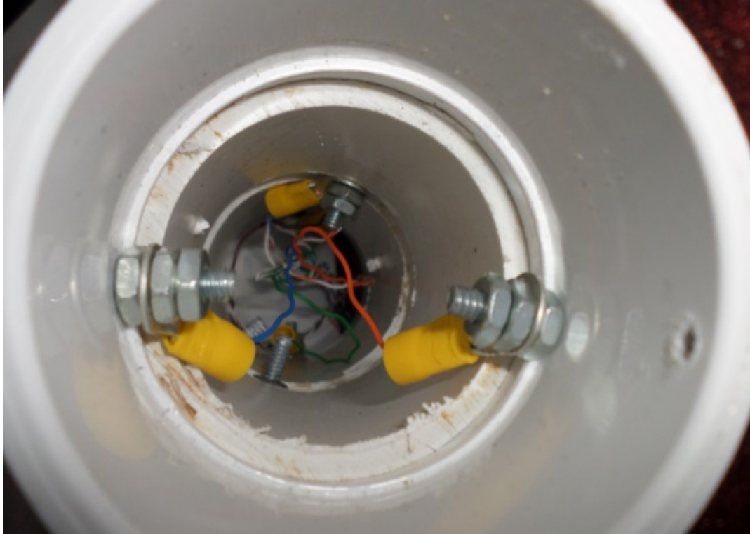
RANGER prop build photo #35: Inside view of the three 2-inch couplings. One ring terminal to the common ground, four to test points, three wires not used. Test point A, the blue wire, is on the left. Test point C, the orange wire, is on the right.
