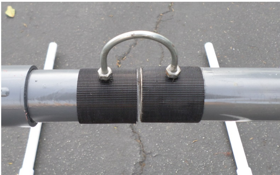
RANGER prop build photo #19: Close up of a #310 U-bolt through both ends of pipe
