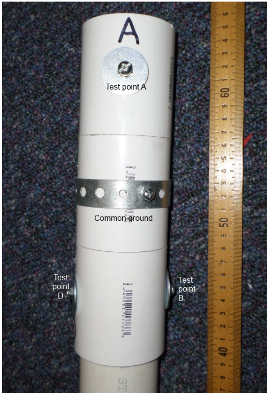
RANGER prop build photo #33: Three 2-inch couplings with a common ground in the center and two test points on either side of the common ground. Note Test point C is on back side of pipe.
