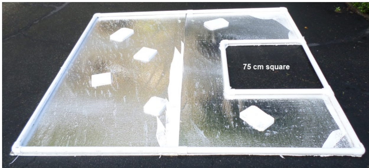
RANGER prop build photo #2: Upside down ice sheet showing framework with foam sheet attached. Note the extra foam used a bottom contours.
