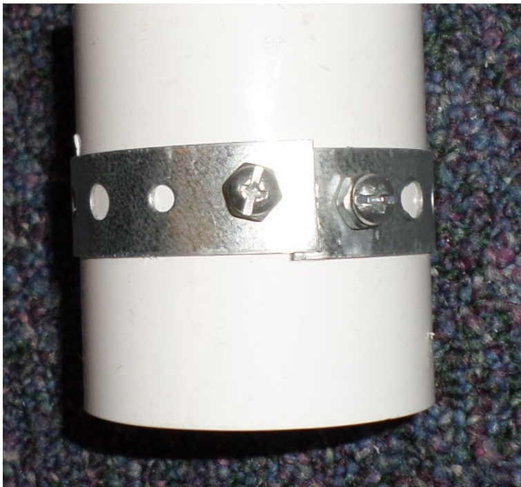
RANGER prop build photo #30: Galvanized hanger strap around middle of 2-inch PVC coupling.
