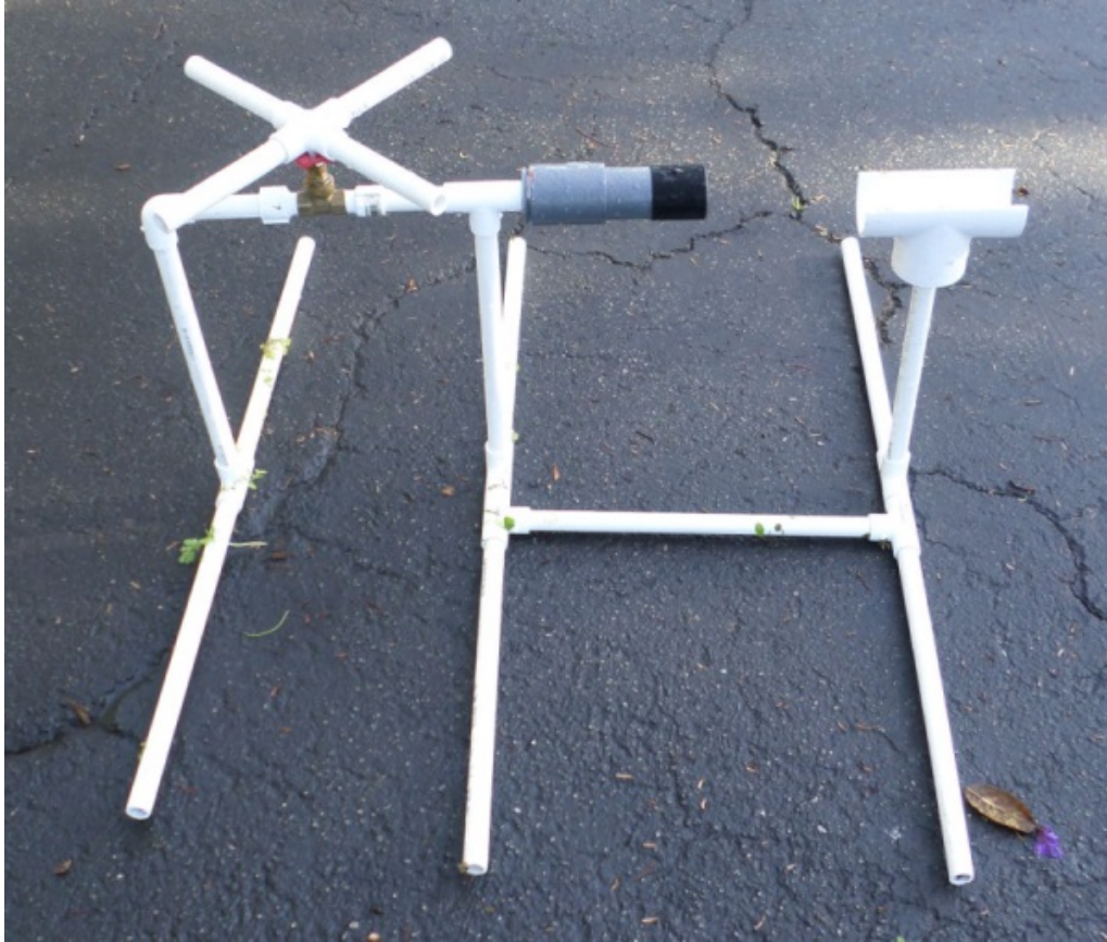
RANGER prop build photo #12: Outer stand with valve handle on end. Note the gray 1 ½-inch pipe.
