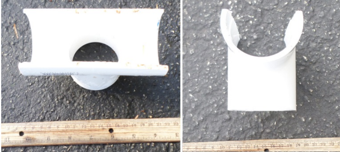
RANGER prop build photo #9: 2-inch tee cut in half lengthwise.
