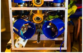
to use two blade instead of three blade for many reasons. The three bladed propellers exert a thrust 5.78 newtons, while the two bladed exert a thrust of 5.33 newtons. The three bladed propeller draws 5.8 amp  $\approx$  12 volts compared to the two bladed which only draws 5.2 amps when running wide open. Our ROV is small, so it doesn't need the extra thrust the three bladed has to
