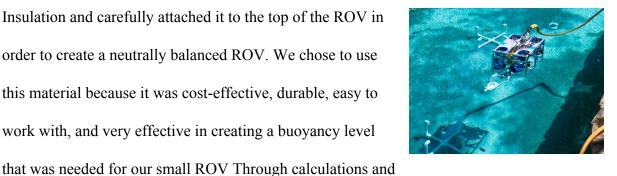
trial and error, we positioned the Foamular R-5 Insulation equally on the top of the ROV and covered up the top wiring with a small rectangle of the material. Additionally, due to the tether slot on the ROV being placed on top, there was a tendency for the tether to dip and pull the ROV in an awkward way. We combated this with cutting out 8 small blades of the Foamular R-5 insulation, which was attached in equal intervals along the tether, thus creating less of a drag on the ROV.
