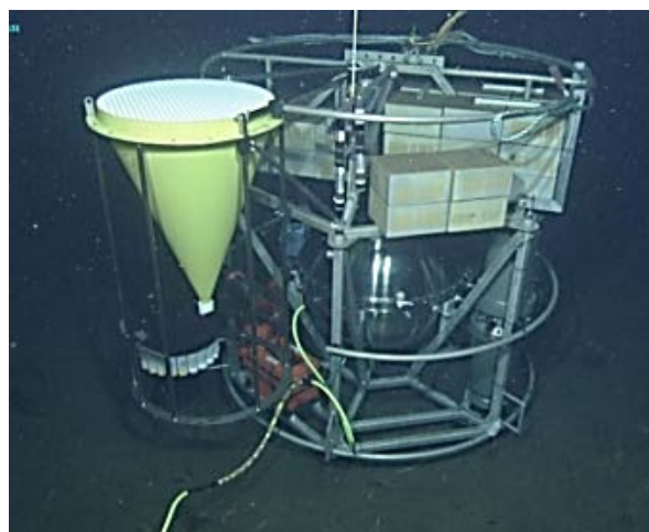
An ESP being prepared for deployment and later connected to the MARS (Monterey Accelerated Research System) cabled observatory, 900 m deep in Monterey Bay. Photo credit: Monterey Bay Aquarium Research Institute, Moss Landing, CA.
