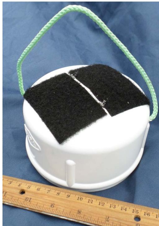
SCOUT product demonstration build photo #2: The wellhead cap.
