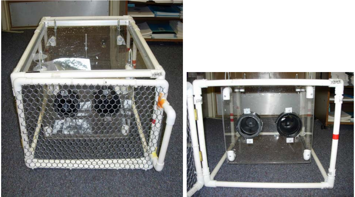
Figure 6: Central node, front view with door closed and door open to reveal ports.
