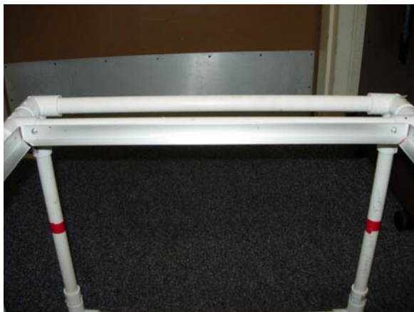
Figure 5: Trawl-resistant frame, view of angle aluminum guide rail.
