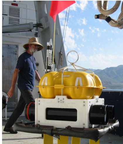
The real thing – an OBS designed and built by Scripps engineers
