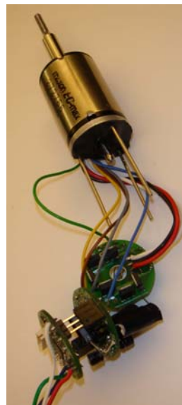
Figure 19 – Custom Motor Controllers
