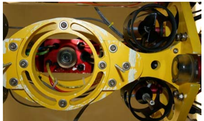
FIGURE 5 – BOTTOM VIEW OF ROV SHOWING INTEGRATED MATING SKIRT AND DUAL CAMERAS FOR TASK #4. THE HATCH SPANNERS FOR TASK #2 ARE ALSO SHOWN
