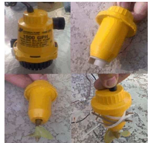
Figure 6 - Process of converting bilge pumps to thrusters (Courtesy of Edgewater High School 2008 Technical Report)
