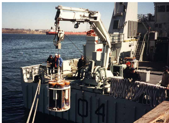
Figure 19: ODIM Brooke Ocean's LARS gets ready to launch a set of ELSS pods.
