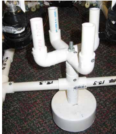
Figure 9: Transfer skirt (bottom) and quad turner (top)
