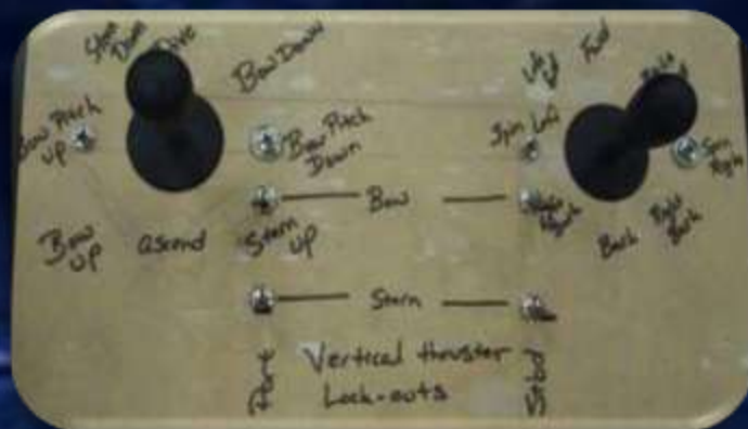
(Figure 17) Control System used for the New England Regional (Currently being cosmetically improved)
