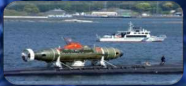
(Figure 27) The Mystic (DSRV 1) attached to a submarine
