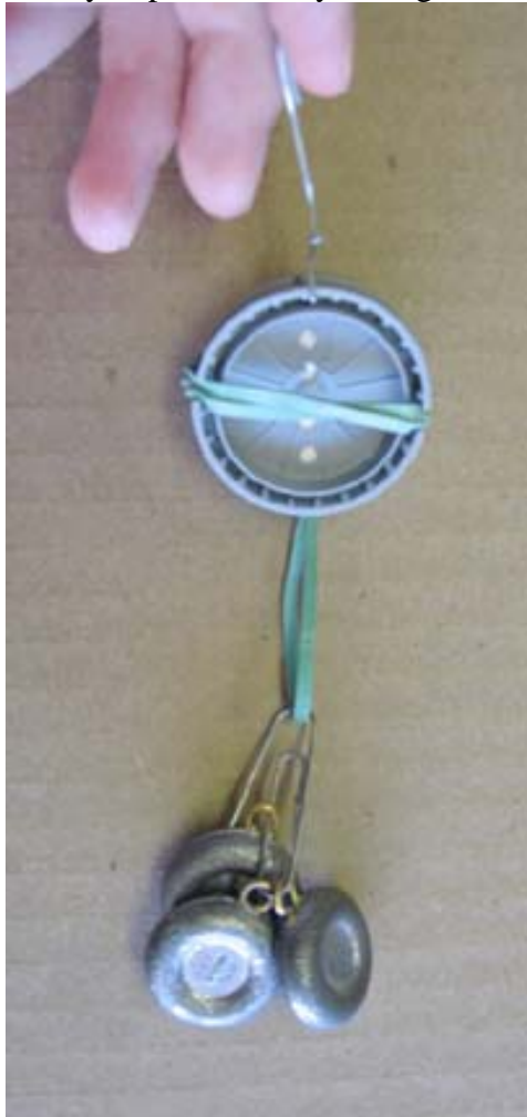
Fig 7. Anchor weights attached to rubber band of release.
