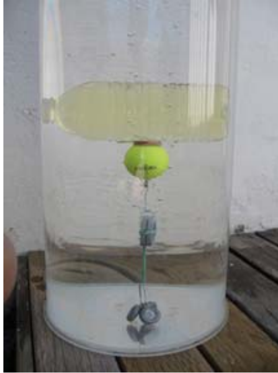
Fig. 3: A working model of the bathyscaphe, demonstrating application of differences in density.
