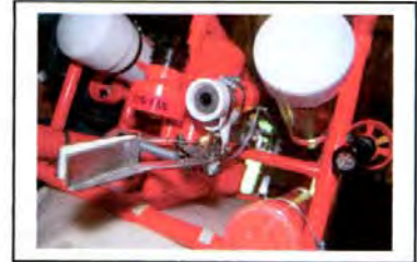
Fig.4-9: Homer's stainless steel universal appendage and attached lipstick camera.
