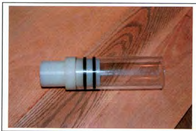
Fig. 4-5 & 4-6: Machining our acrylic brushless motor housings and the finished product. The white portion is machined from nylon for its' lightweight and strength.
