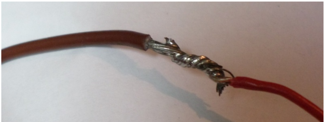
Photo #3: Two wires soldered together. Note the outline of the individual wires is still visible under the solder.
