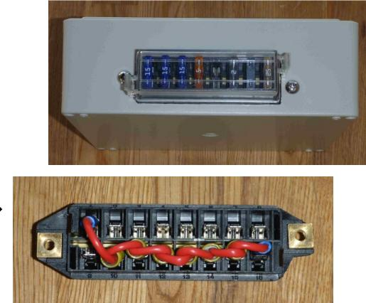
Note: The jumper marked by the arrow is an error. It does not connect to the primary fuse. It should be long enough to connect to the main power switch output.
