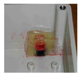
**Fuse block-** Mark a rectangular hole in the back of the box for the fuse block. Keep the hole low, at the bottom edge of the box. This design is for an 8 circuit fuse block. Use a dremel style tool to remove the plastic material. Shape the hole with a medium file and install the fuse block.
