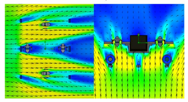
What can be interpreted from this? The ROV has the least amount of drag in the forward motion, just as it was wanted. The sideway and down drags are much bigger, but the sideways drag does not make that a big
