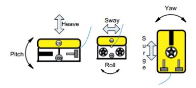
The maximum allowance in the budget is six thrusters. There are different methods to place the thrusters in order to get the five DoF and three of them have been evaluated. The different method is shown at the picture below. It has been decided to have six thrusters in total due to the total power. Both method B and C have six thrusters but due to the current limit set by MATE, the method B is a better choice because in method C the power of the thrusters will not be fully utilized.
