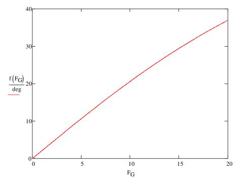
The maximum angle for the ROV with the maximum force of 20N acting on the gripper:
