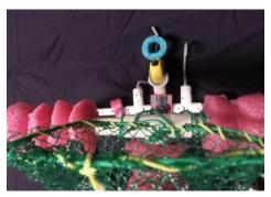
A fruit net was used to keep a long distance from the back of the net to the frame so the algae would float up but be kept in the net. Since the net is at the top of the ROV, it is not visible in the camera. To fix this problem a mirror was placed on the front/bottom PVC pipe at an angle to allow the camera to view the net and its placement compared to the placement of the simulated algae in the mission "Science Under the Ice".
