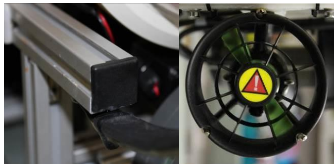
Figure 32: Cover on sharp edge and safety labels are put up on thruster
