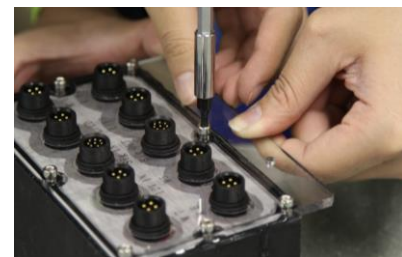
Figure 14: Waterproofed box containing 7 ESCs
