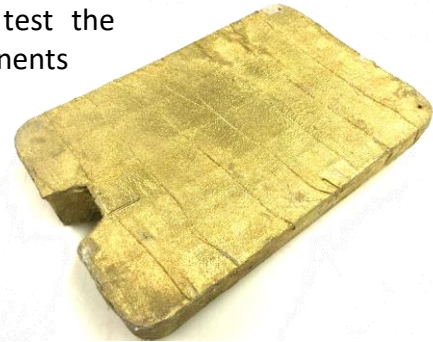
Figure 16: Styrofoam providing 30N of buoyancy
