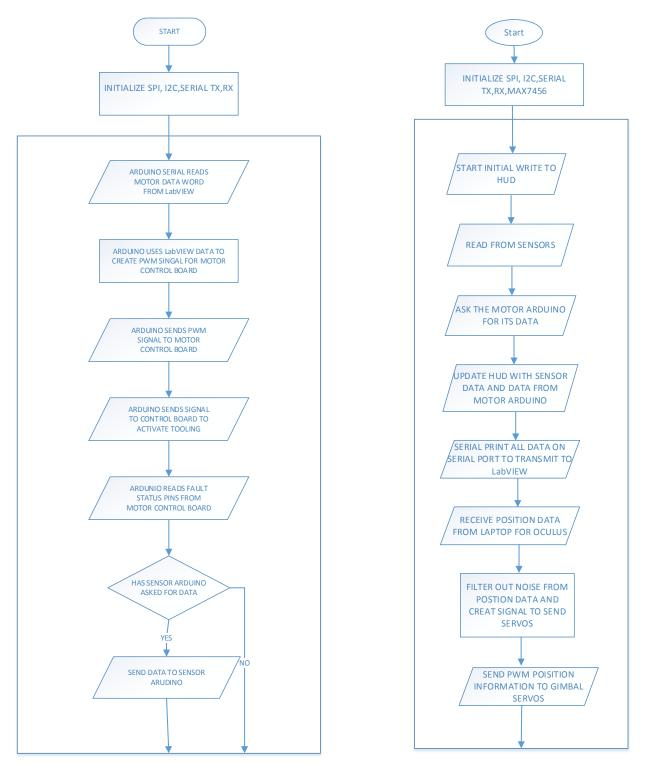
FIGURE 5 FLOWCHART SHOWING THE SOFTWARE FLOW OF THE ARDUINOS. MOTOR ARDUINO ON LEFT, SENSOR ARDUINO ON RIGHT
