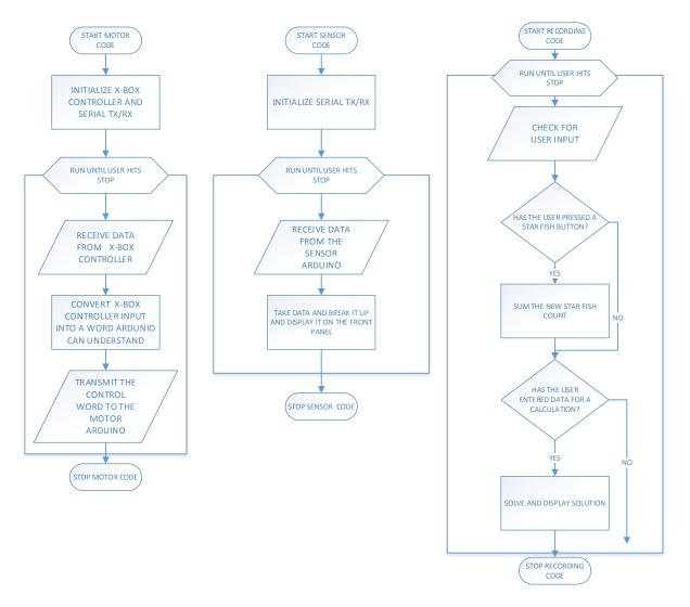
FIGURE 6 FLOWCHART SHOWING THE THREE MAIN LOOPS OF THE LABVIEW CODE
