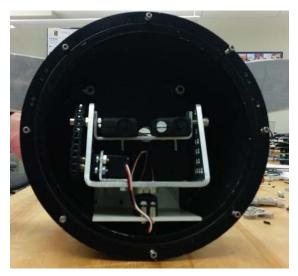
FIGURE 4 THIS PHOTO SHOWS THE MOBIUS ACTIONCAM'S MOUNTED ON THE GIMBAL IN THE CAMERA HOUSING
