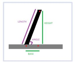
FIGURE 7 ARTIST INTERPRETATION OF THE LASER'S BEING USED TO DETERMINE THE LENGTH AND ANGLE OF THE WELLHEAD. PURPLE INDICATED CALCULATED VALUES, GREEN INDICATED MEASURE VALUES
