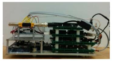
FIGURE 8 THIS PHOTO SHOWS A SIDE VIEW OF THE SHELVING SYSTEM DEVELOPED TO SAVE SPACE INSIDE THE MAIN HOUSING
