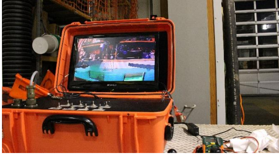
The main topside control case at a pool test
