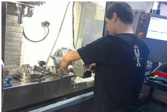
Nicholas machining an end cap for the WEC
