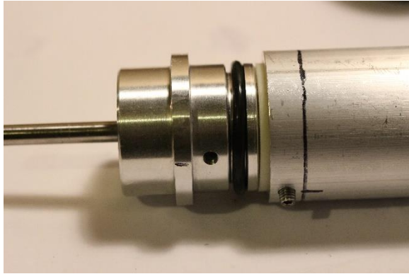
The machined manipulator sealing system
