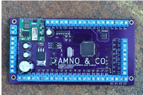
The custom PCB for topside communications
