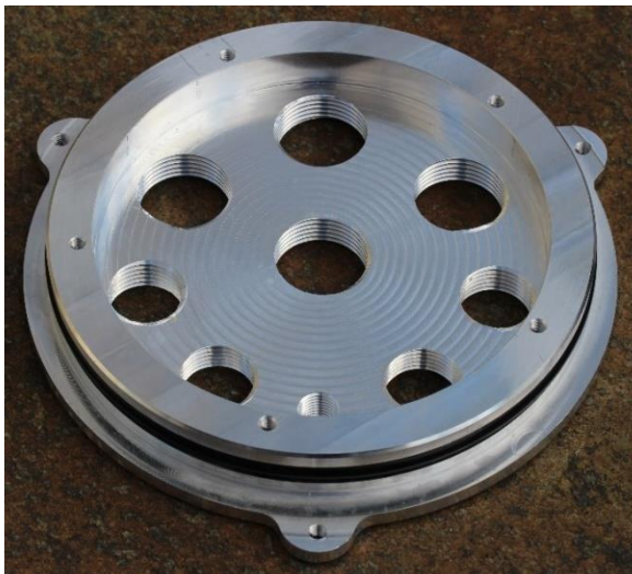
The rear end cap to the WEC
