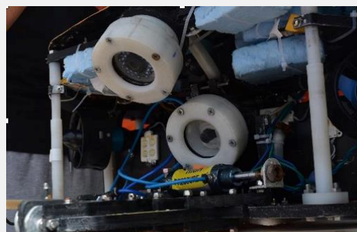
Figure 13. Cameras mounted on Triton ROV after fabrication.
