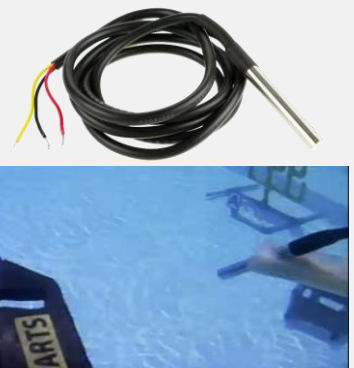
Figure 28. Temperature sensor before and after installation.
