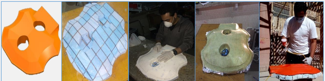
Figure 14. Fiber Glass Fabrication Process.
