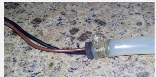
Figure 11. Wire sealing technique
