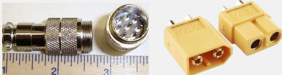
Figure 16. Polarized 8-pin connector on the left and XT60 power connector on the right.
