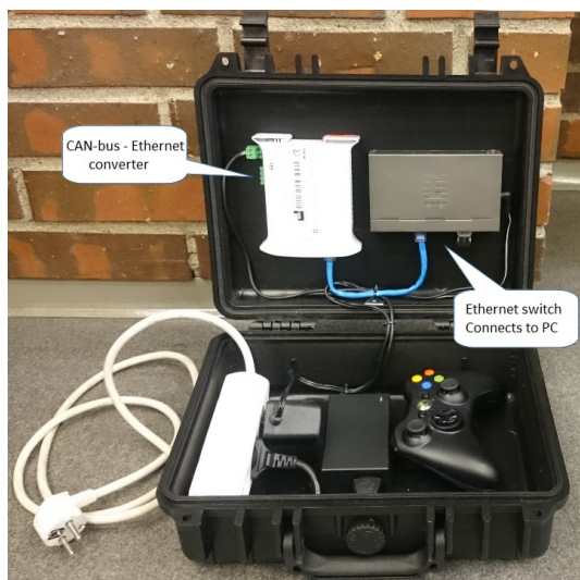
Figure 2.10: Plastic case used at surface as interface between control system and Ægir.
