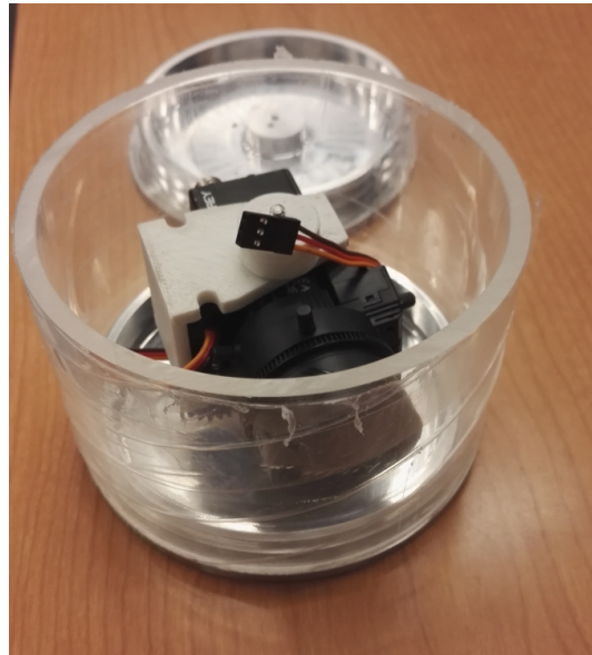
Figure 2.9: Main camera housing, with IP-camera mounted together with a small servo for tilt control.
