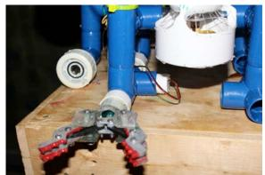
Figure 4: The Manipulator's fingers, with red tips (Photo: R. McClary)
