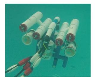
Figure 7: The backside of the FDS 2016 showing the four top ballast tubes that keep the vehicle stable underwater. (L. Potter).
