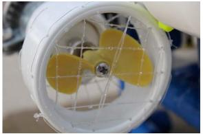
Figure 3: The Kort nozzles with safety netting (Photo: R. McClary)
