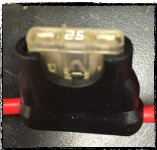
Figure 16: 25A fuse in the control system wiring.
