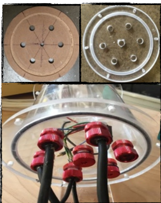
Figure 7: Wooden draft of housing cover (left). Final acrylic cover (right). Waterproofed connectors attached to the cover (bottom).
