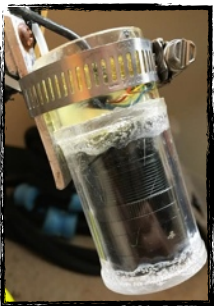
Figure 9: Camera housed in waterproofed acrylic tube.
