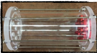
Figure 5: Honu's on-board electronics housing.
