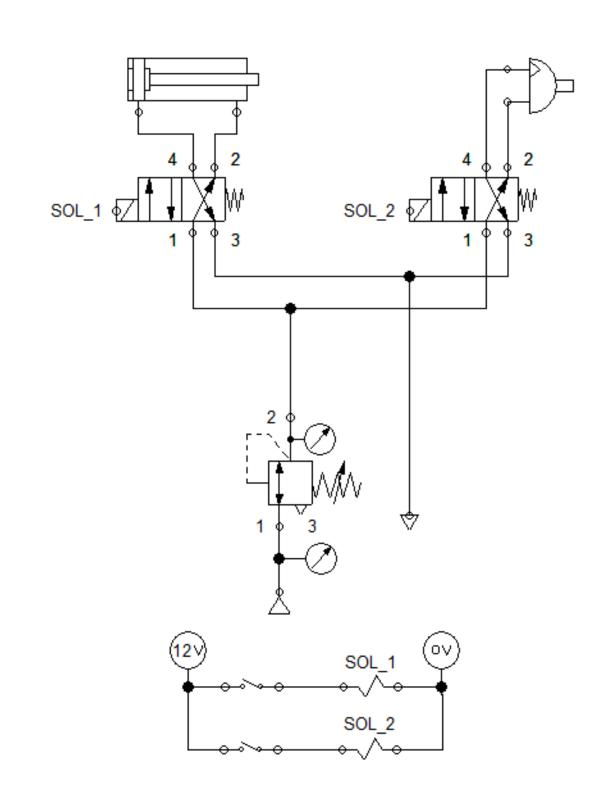
Pneumatics system enabling the claw function of the ROV
