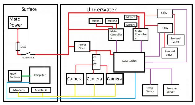
Electronic System of the ROV enabling movement
