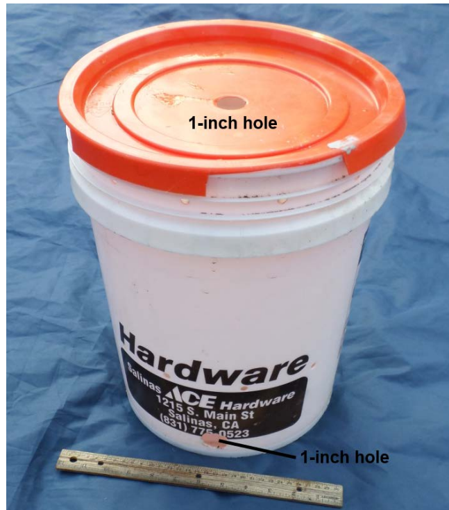
EXPLORER product demonstration build photo #1: 5-gallon bucket with hole drilled through the side wall. 5-gallon bucket lid with hole drilled into center.
