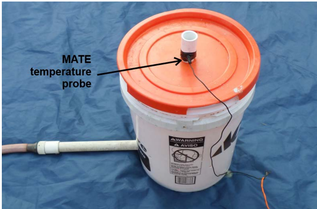
EXPLORER product demonstration build photo #3: Completed vent structure with MATE temperature probe inserted into the pipe.
