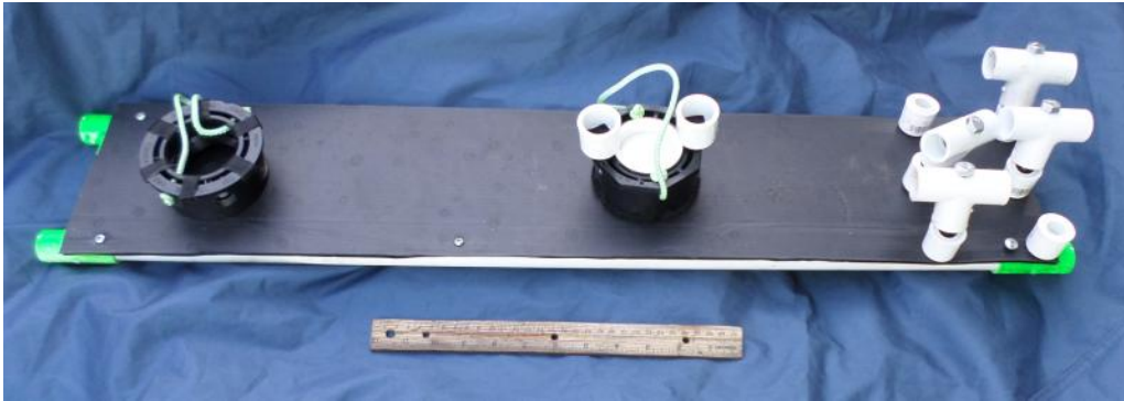
RANGER product demonstration build photo #34: The elevator holding one flanges, one wellhead cap and four bolts.
