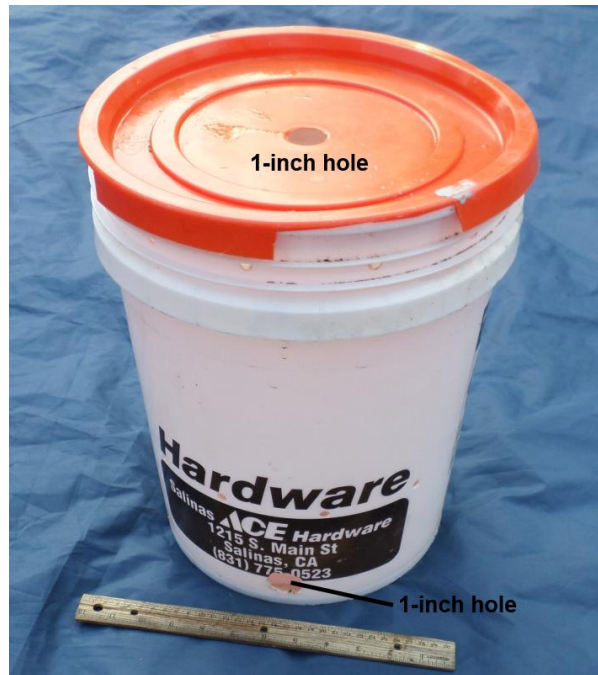
RANGER product demonstration build photo #1: 5-gallon bucket with hole drilled through the side wall. 5-gallon bucket lid with hole drilled into center.
