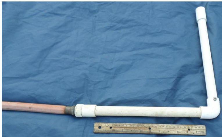
RANGER product demonstration build photo #2: Water bearing ¾-inch pipe.
