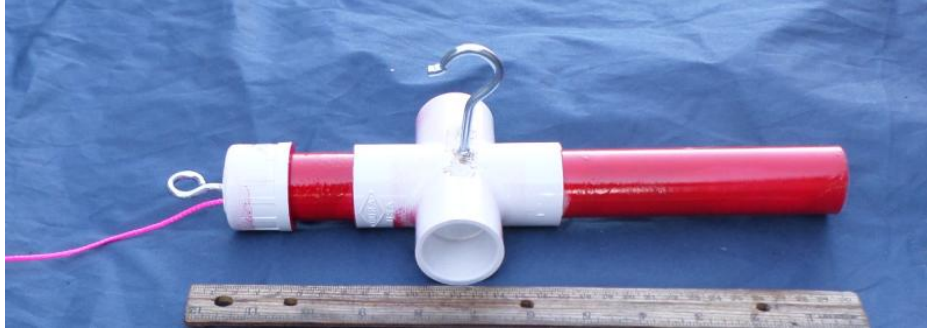
RANGER product demonstration build photo #8: The cable connector.
