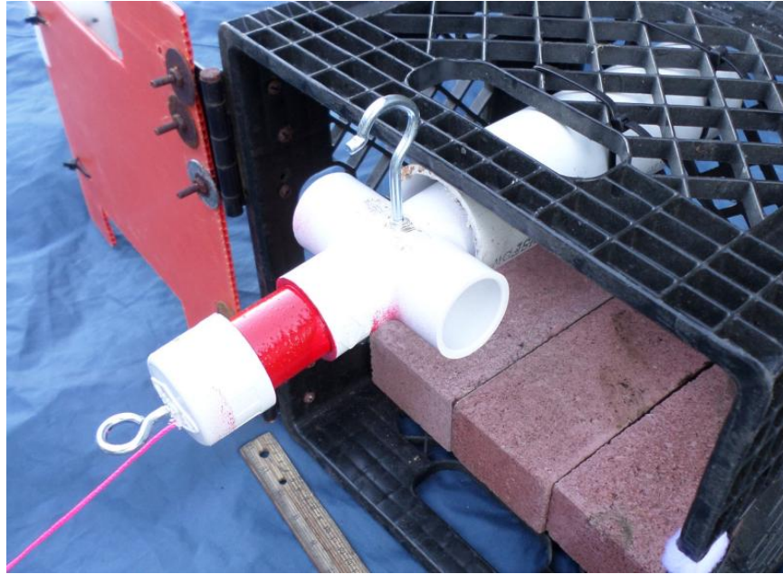
RANGER product demonstration build photo #12: The cable connector successfully inserted into the port on the power and communications hub.
