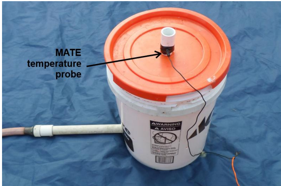
RANGER product demonstration build photo #3: Completed vent structure with MATE temperature probe inserted into the pipe.
