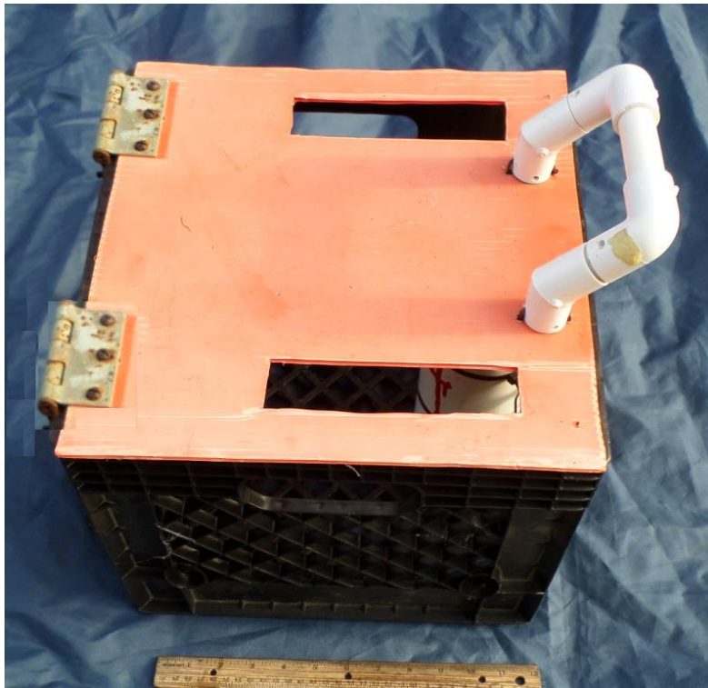
SCOUT product demonstration build photo #5: The power and communications hub with the door closed.
