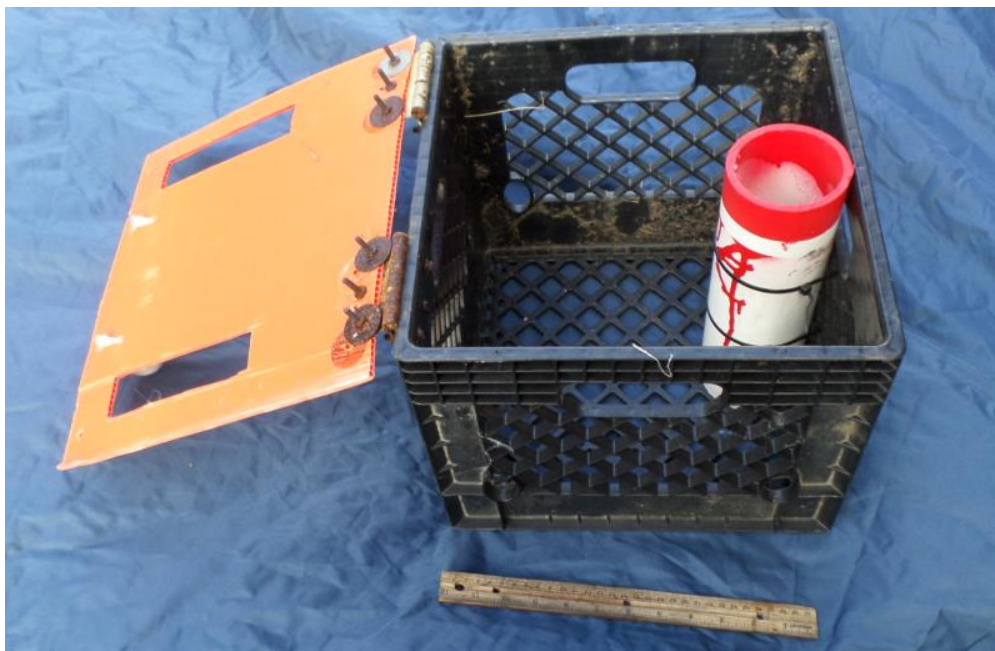
SCOUT product demonstration build photo #6: The power and communications hub with the door opened, exposing the 3-inch port.
