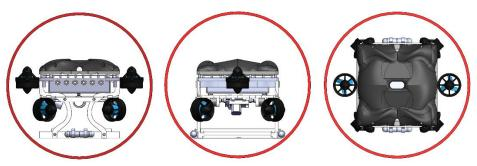
Figure 3: CAD Rendering of Vimy with a 580 mm Diameter Circle in Each Axis
