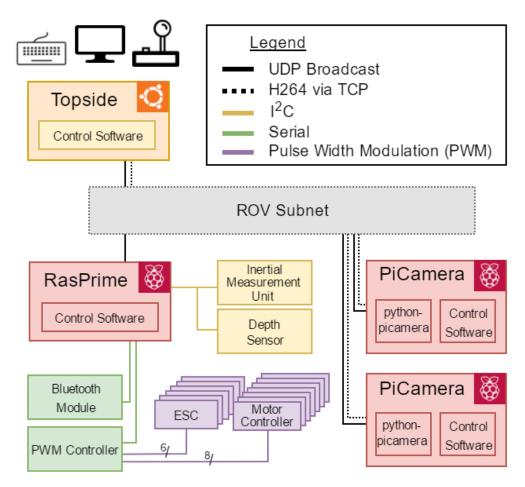
Figure 16: Software Communications Block Diagram
