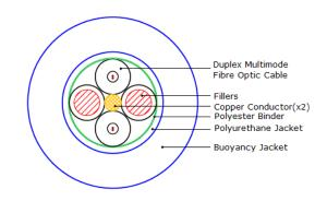
Figure 14: Tether Cross Section View
