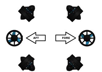
Figure 6: CAD Rendering of Thruster Layout
