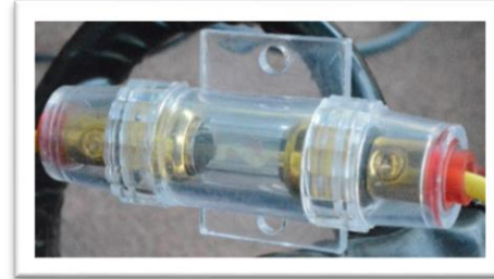
Figure 26: 30 A fuse in acrylic fuse holder
