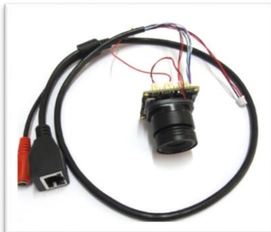
Figure 16: IP Board camera with SONY lens
