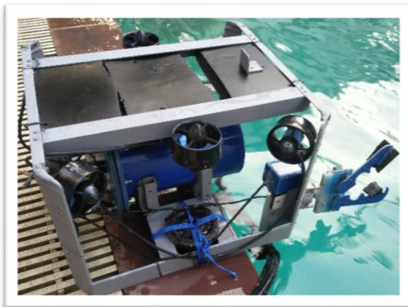
Figure 6: EVA foam mounted on Mansarover for buoyancy
