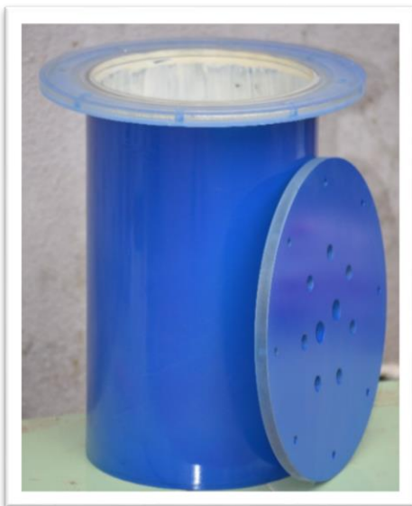
Figure 3: Acrylic Electronic Chamber painted blue.
