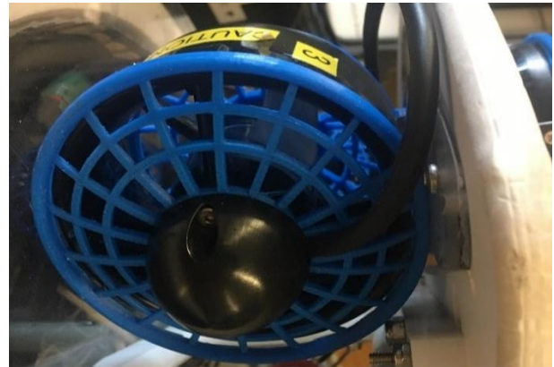
Figure 7: 1 of 6 BlueRobotics™ T100 Thrusters on ICE
