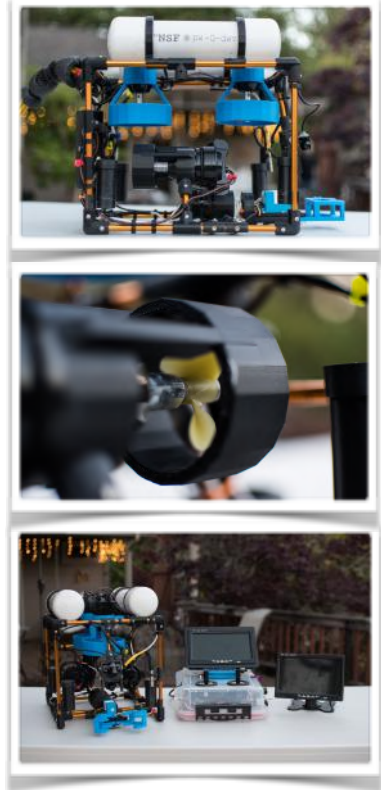
Top: Side view of the Argo IV. Middle: A 500 gph motor with a shroud for safety. Bottom: The Argo IV, the monitor and control box, and the second monitor.
