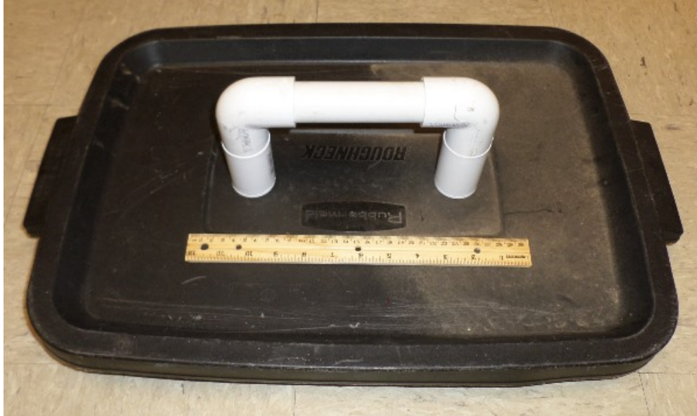
EXPLORER build photo #37: Cap with 1-inch PVC handle.
