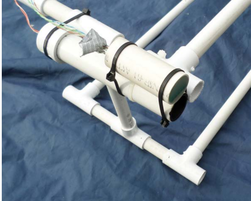
EXPLORER build photo #47: The RFID port and Bluetooth Master module cylinder mounted on a container.
