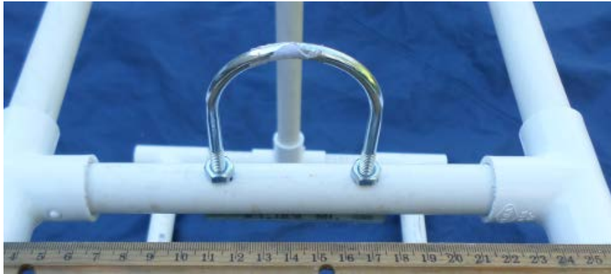
RANGER build photo #40: U-bolt installed at the top, center of the container.
