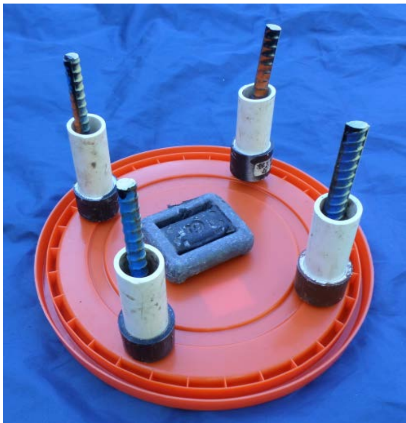
EXPLORER product demonstration build photo #5: Four lengths of rebar installed on the elevator.
