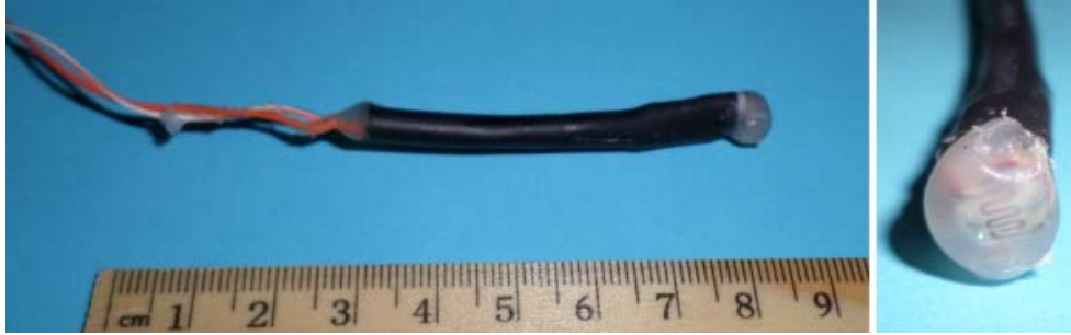
EXPLORER build photo #43: Sealed and waterproofed light sensor.
