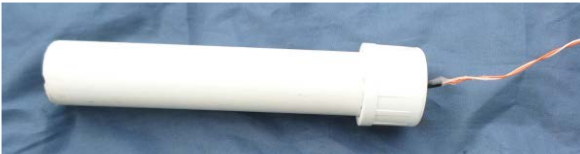
EXPLORER build photo #45: Port with light sensor positioned 15 cm down length of pipe.
