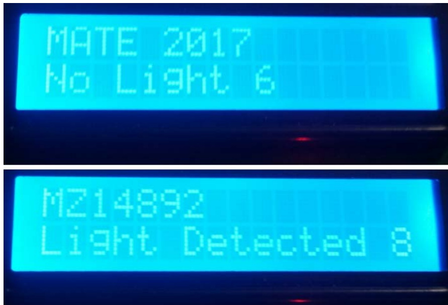
EXPLORER build photo #48: Display shields showing the base message and the container ID number.
