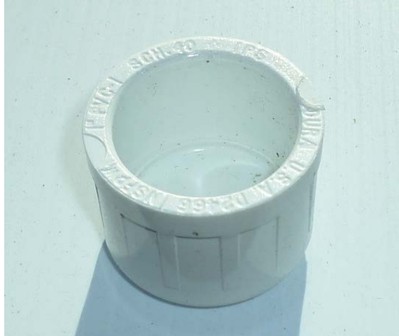
EXPLORER product demonstration build photo #28: 1-inch end cap holder for fountain.
