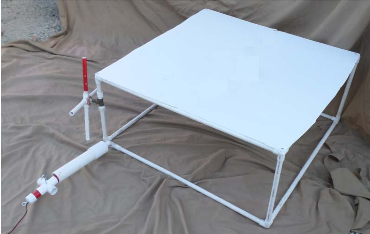
NAVIGATOR product demonstration build photo #7: Corrugated plastic sheet on top of the platform framework.
