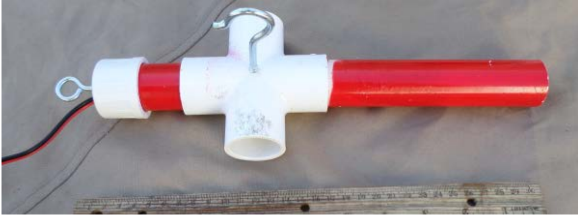
NAVIGATOR product demonstration build photo #2: The cable connector.
