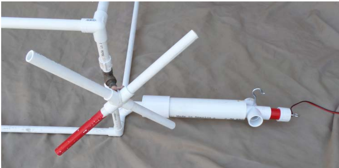
NAVIGATOR product demonstration build photo #6: The valve attached to the platform framework with the power cable connector installed.
