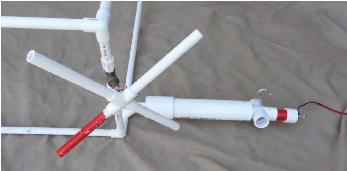
NAVIGATOR product demonstration build photo #22: The valve attached to the platform framework with the power cable connector installed.
