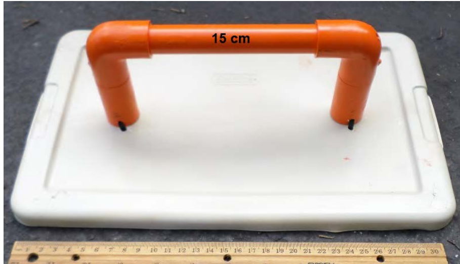
NAVIGATOR build photo #31: Cap with 1-inch PVC handle.
