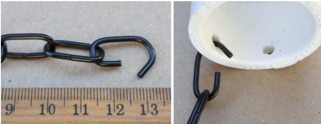
NAVIGATOR product demonstration build photo #8: Opened chain link and the opened chain link through the coupling.
