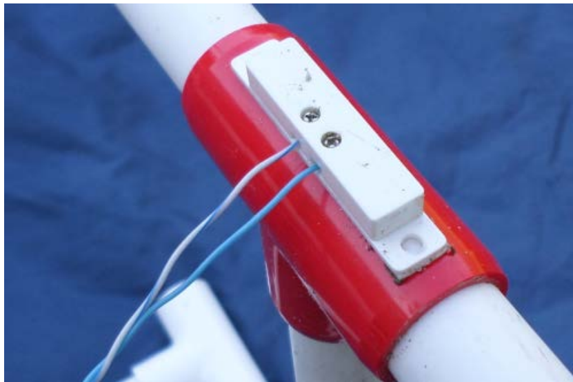
NAVIGATOR build photo #37: Magnetic reed switch mounted on container.
