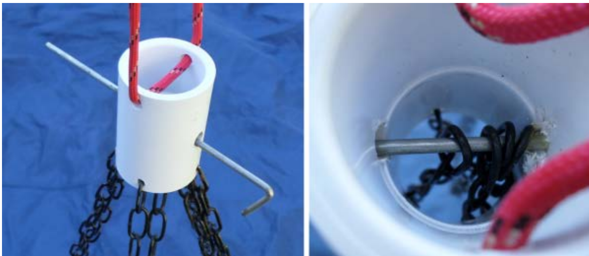
NAVIGATOR product demonstration build photo #13: All four chains held in place in the coupling.
