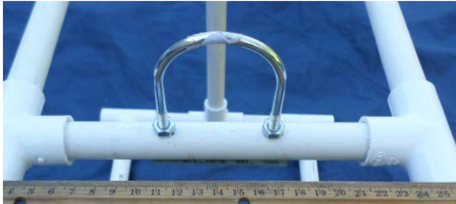
NAVIGATOR build photo #34: U-bolt installed at the top, center of the container.
