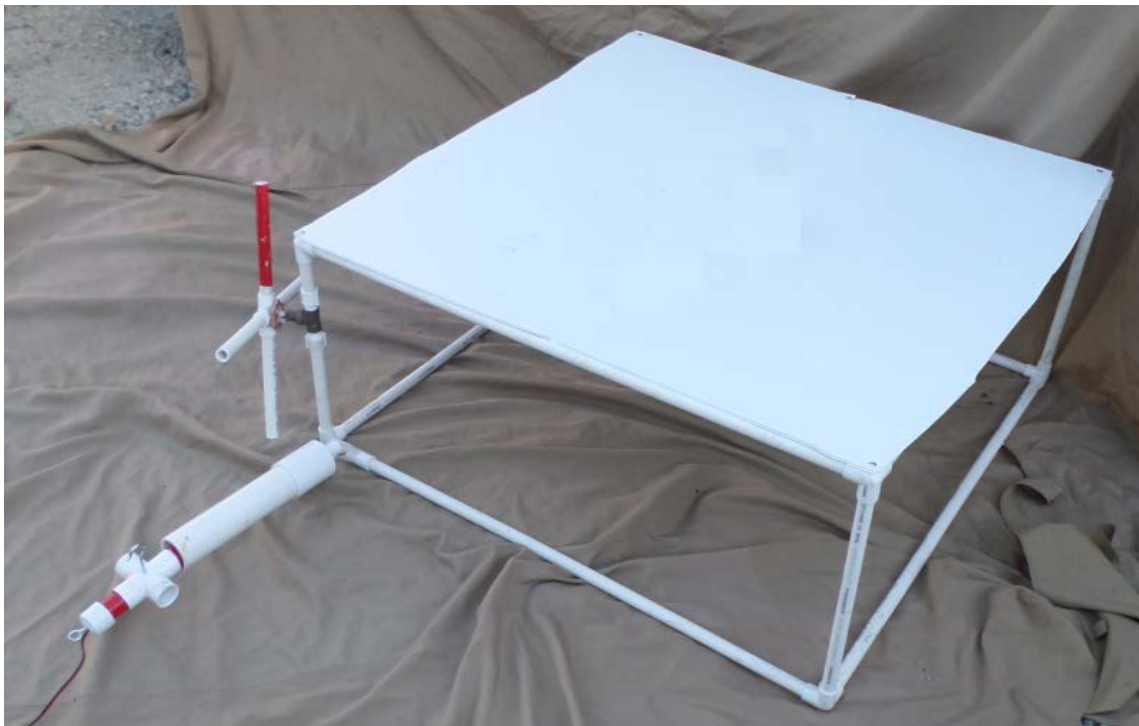
NAVIGATOR product demonstration build photo #23: Corrugated plastic sheet on top of the platform framework.
