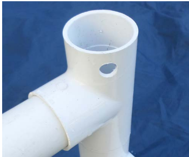
NAVIGATOR product demonstration build photo #10: Hole in the inside top of the frame.
