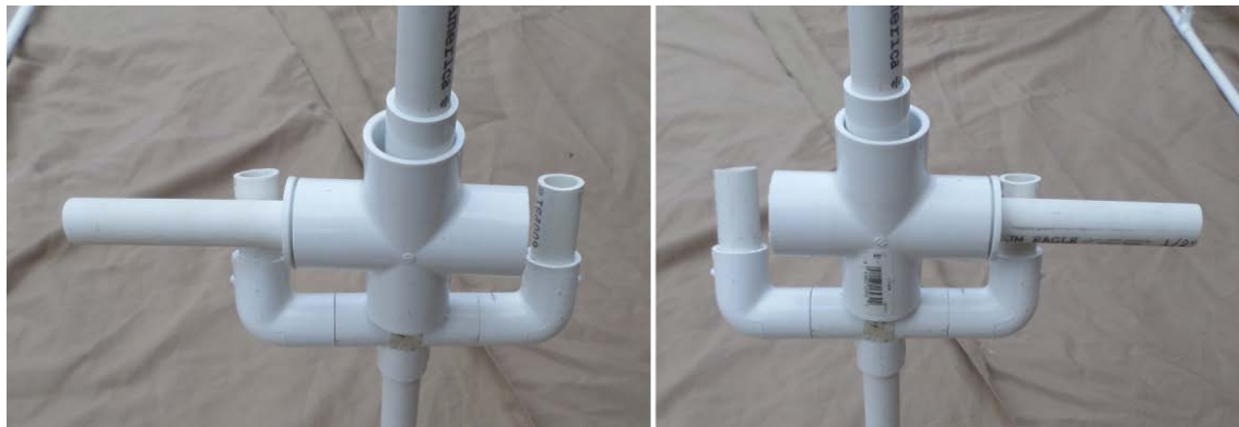
RANGER product demonstration build photo #7: Locking mechanism; locked (left) and unlocked (right).
