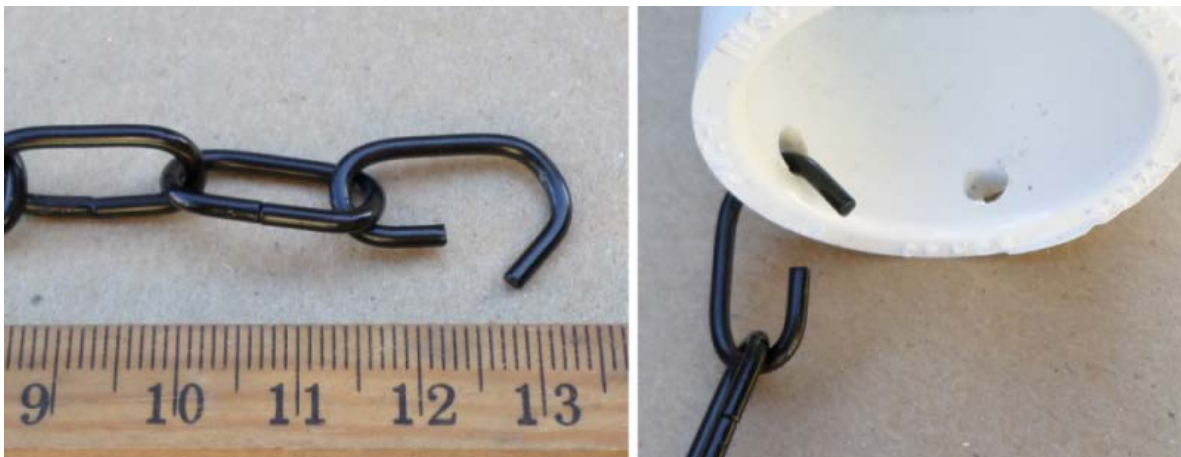
RANGER product demonstration build photo #8: Opened chain link and the opened chain link through the coupling.
