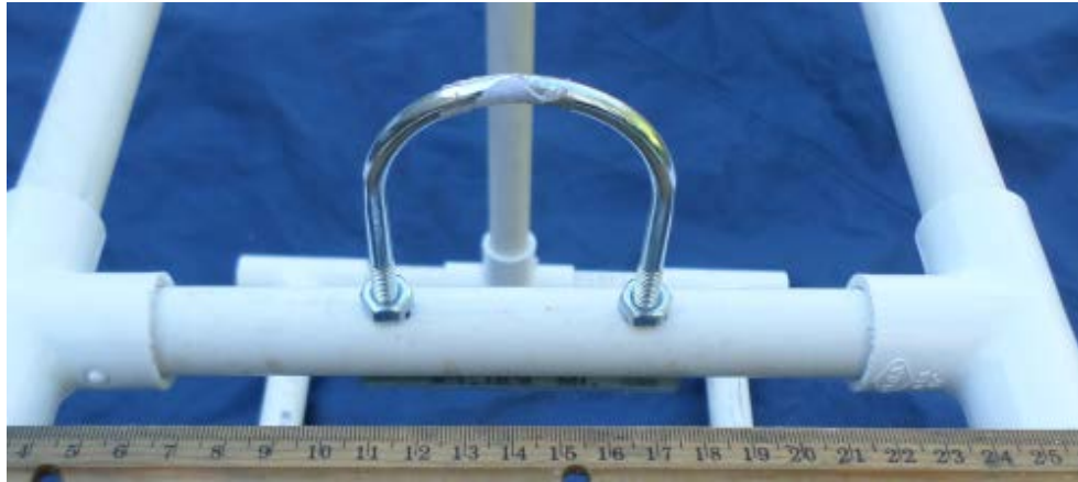
RANGER build photo #44: U-bolt installed at the top, center of the container.
