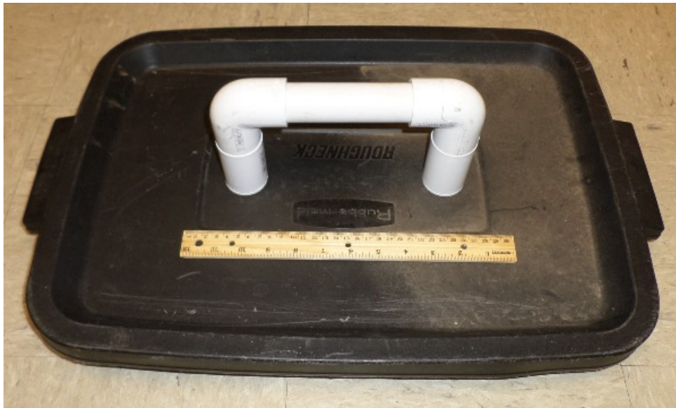
RANGER build photo #41: Cap with 1-inch PVC handle.
