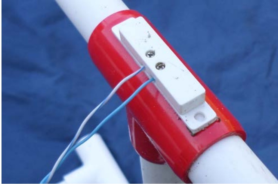
RANGER build photo #48: Magnetic reed switch mounted on container.
