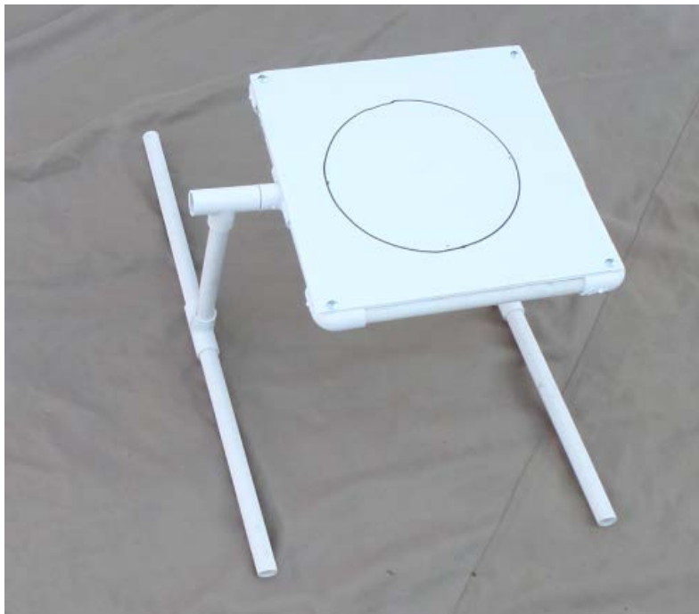
SCOUT product demonstration build photo #6: Corrugated plastic on framework.
