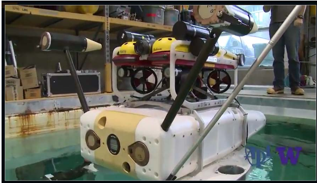
The Saab Falcon ROV deploying the I-AMP in the UW test tank.
