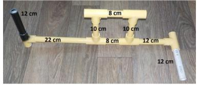
The 12 cm black handle should be parallel (in line with) the central yellow section.
