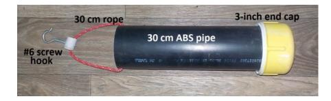
Drill two holes on opposite sides of the bottom of the lift bag. String 30 cm of rope through the holes. Run the rope through the 2 cm long length of pipe with the screw hook attached.
