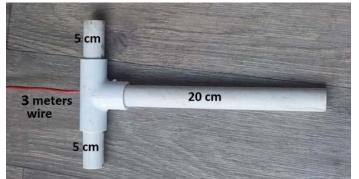
Drill a hole into the top of the ½-inch tee. Tie an overhand knot in the wire to secure it inside the tee.
