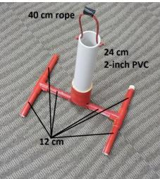
A 40 cm length of rope at the top of the 2-inch PVC can be used as a grab point for moving the base into the designated area.
