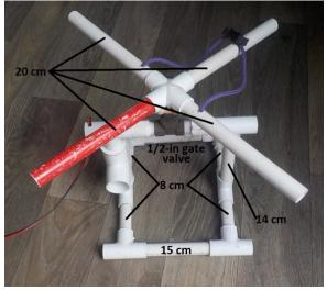
Flotation will be added into the PVC of the handle to make the OBS weight less than 5 Newtons in water.
