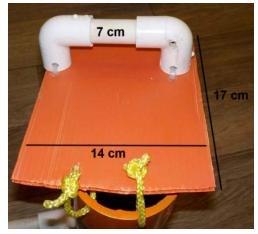
Two 20 cm of <u>rope</u> (colors may vary) are used to attach the door to the top of the hub. The door is 17 cm by 14 cm.
