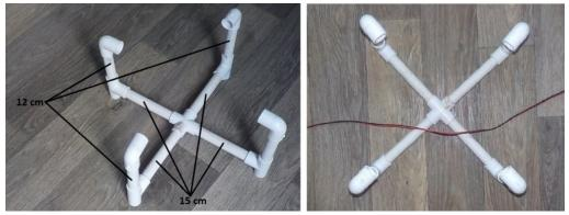
The cable must go through two "legs" of the waypoint. The photo on the right shows the cable through two "legs" of the waypoint.
