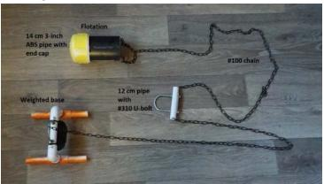
The length of the mooring from the bottom of the base to the top of the flotation should be the depth of the pool plus 5 to 10 cm.
