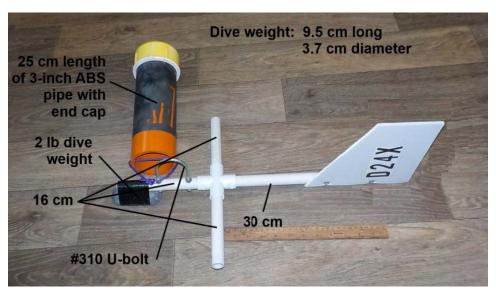
The 25 cm of 3-inch ABS pipe with PVC end cap is positively buoyant and will float approximately 15 cm above the bottom of the pool. If ABS pipe is not available in your area, PVC pipe can be substituted. However, additional flotation may need to be added to make the lift bag positively buoyant in water. For example, 3-inch PVC pipe may need to be cut to a longer length (longer than 25 cm) to compensate for the additional weight of the pipe in water.
