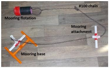
The mooring attachment should be approximately half way between the base and the flotation. Cut your chain lengths accordingly.
