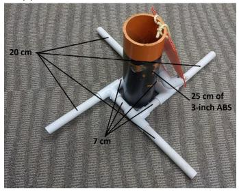
Use 2-inch screws to attach the 3-inch ABS pipe to the PVC base. The screws will go through the ½-inch pipe and into the base of the 25 cm length of 3-inch ABS. Note: 3-inch PVC pipe can be substituted for ABS pipe.
