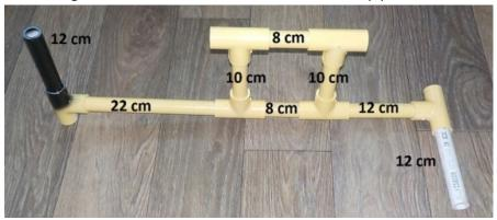
The 12 cm black handle should be parallel (in line with) the central yellow section.
