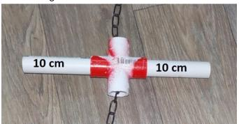
Drill a hole in opposite ends of the ½-inch cross (two holes total). Use needle nose pliers to open the chain links on the ends of the chains attached to the mooring flotation and the mooring base. Insert the open link for the chain leading to the flotation on one side. Insert the open link for the chain leading to the base on the other side of the cross. Use the pliers to push the link back together.
