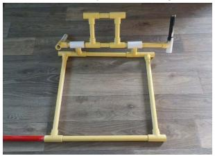
The ½-inch pipe of the locking mechanism fits through the ¾-inch sections of the tees.
