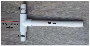
Drill a hole into the top of the ½-inch tee. Tie an overhand knot in the wire to secure it inside the tee.
