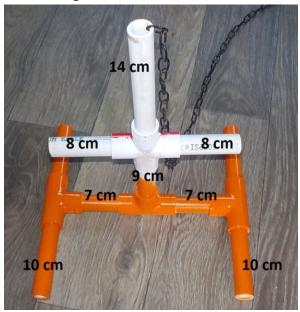
Drill a 1/8-inch hole in the top of the 14 cm length of pipe. Use needle nose pliers to open one link of the chain, insert it through the drilled hole, then push the chain link back together.
