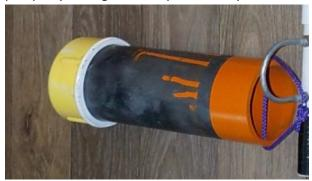
Drill two holes on opposite sides of the bottom of the lift bag. String 30 cm of rope through the holes and tie the ends of the rope together through the #310 U-bolt.
