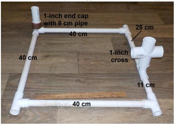
Screw the 1-inch end cap into the tee at corner of the elevator.
