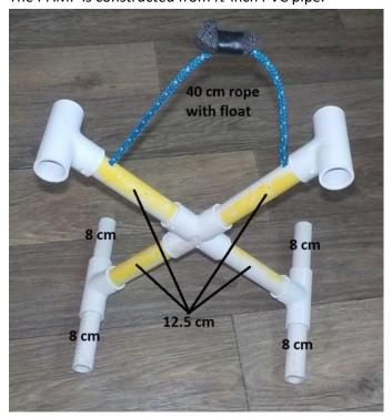
40 cm of <u>rope</u> (colors may vary) is used as a grab point. Drill two holes 0.5 cm below the tees. Insert the rope into the holes and tie an overhand knot to secure the rope in the pipe.
