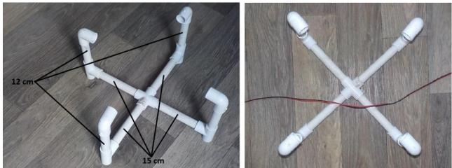
The cable must go through at least one "leg" of the waypoint. The photo on the right show the cable through two "legs" of the waypoint.
