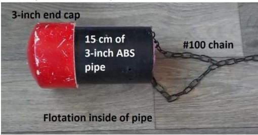
The mooring is constructed from a 15 cm length of 3-inch ABS pipe and a 3-inch PVC end cap. PVC pipe can be substituted for ABS.
