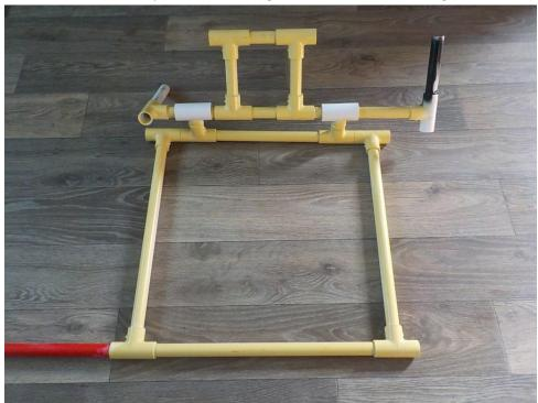
The  $\frac{1}{2}$ -inch pipe of the locking mechanism fits through the  $\frac{3}{2}$ -inch sections of the tees.
