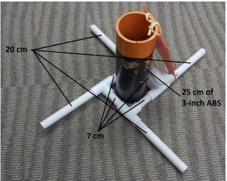
Use 2-inch screws to attach the 3-inch ABS pipe to the PVC base. The screws will go through the ½-inch pipe and into the base of the 25 cm length of 3-inch ABS. Note: 3-inch PVC pipe can be substituted for ABS pipe.
