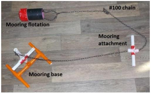
The mooring attachment should be approximately half way between the base and the flotation. Cut your chain lengths accordingly.
