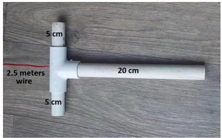
Drill a hole into the top of the ½-inch tee. Tie an overhand knot in the wire to secure it inside the tee.
