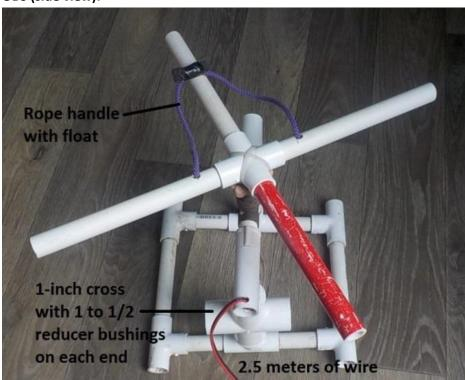
A 40 cm length of <u>rope</u> (colors may vary) may be used as a grab point to move the OBS. The two ends of the rope are approximately 12 cm apart. A small section of foam is attached to center of the rope to provide flotation.
