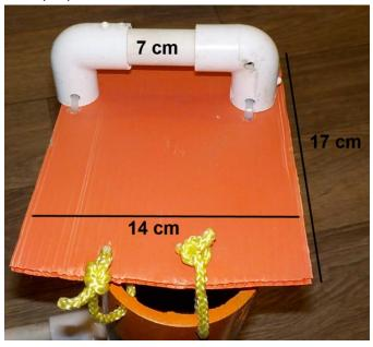
Two 20 cm of <u>rope</u> (colors may vary) are used to attach the door to the top of the hub. The door is 17 cm by 14 cm.
