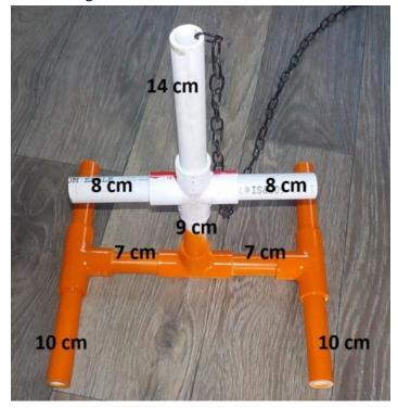
Drill a 1/8-inch hole in the top of the 14 cm length of pipe. Use needle nose pliers to open one link of the chain, insert it through the drilled hole, then push the chain link back together.
