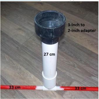
The 33 cm lengths of PVC pipe will attach to the designated area for the I-AMP and the designated area for the mooring (see below).
