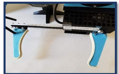
Figure 10: Blue's main actuator intended for grabbing and lifting Credit: Liam Acres
