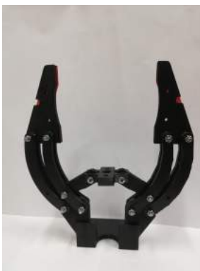
Figure 14: 3D-printed prototype of the manipulator
