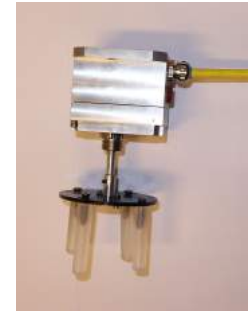
Figure 12: The tool made for leveling the OBS
