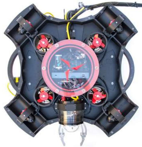
Figure 5: Bird's-eye view showing the thruster layout
