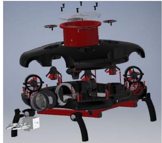
Figure 4: Exploded view of Manta's major parts
