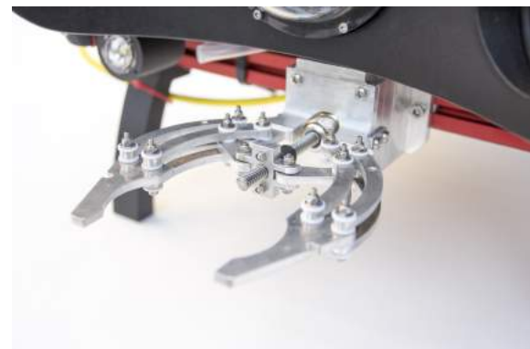
Figure 15: Finished manipulator manufactured in aluminium
