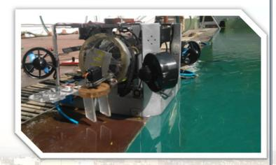
Safety Features: Master Fuse, 3D Printed Thruster Shrouds, Separate Safety checklist for production and off-shore, no sharp edges, Realtime Voltage & Current Monitoring
