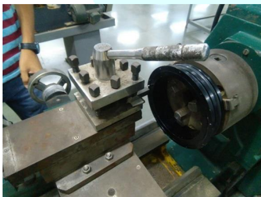
Making grooves for O-ring on Lathe Machine
