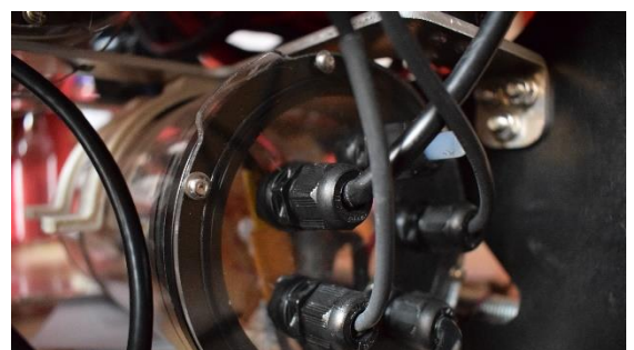
Figure 4 Cable glands used to allow cables into the control box
