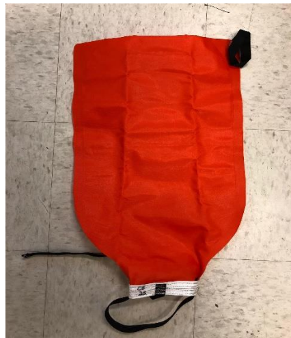
Figure 12: lift bag (designed for 25lb payload)
