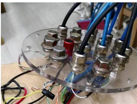
Figure (16) Sturgeon's cables passing through the glands
