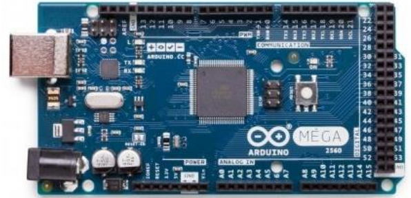
Figure (20) Arduino Mega microcontroller
