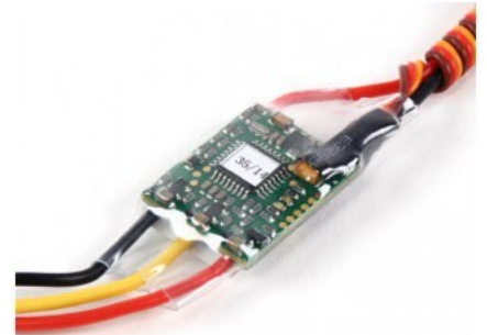
(Above) Blue Robotics ESC's allow the ROV to receive the appropriate signals requires for the ROV to maneuver in the water . Photo courtesy of Blue Robotics.
